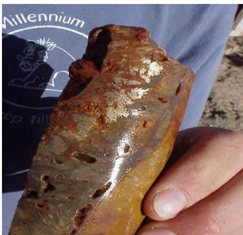
Drill core showing free gold
