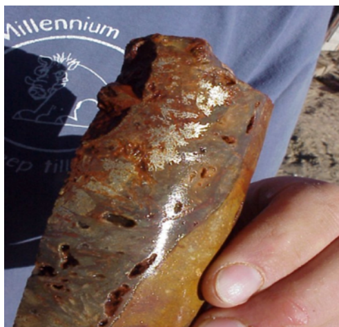
Drill core showing free gold
