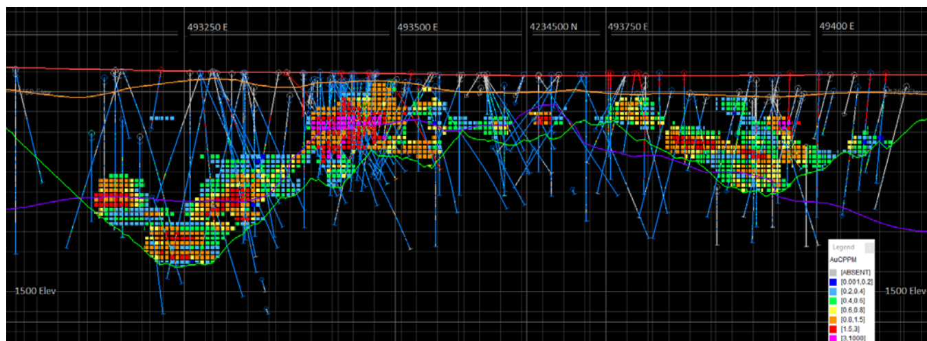
Figure 14-11: Long Section (Looking N20E) view showing drill holes, estimated blocks, and pit shell used to constrain resource estimate.
