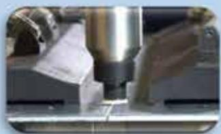
“Transforming materials at the molecular level, Friction stir welding is the silent powerhouse of modern manufacturing”
