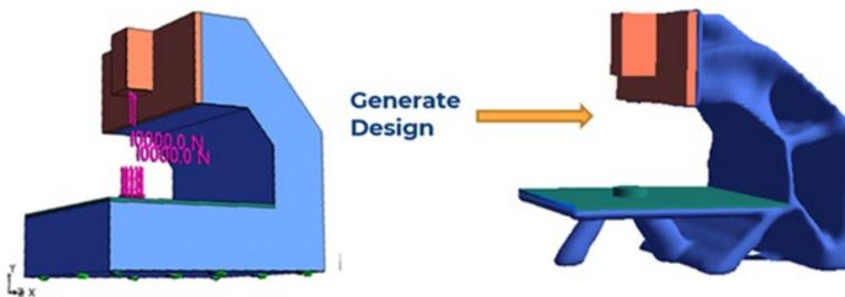
The second step toward the goal is enabling Generative Design of a multiple components simultaneously within an assembly context. The illustration below shows Generative Design of multiple components of the assembly performed simultaneously.
