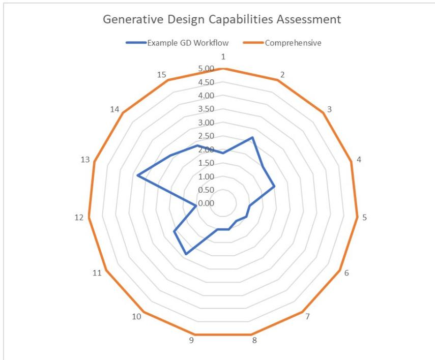
*A Suitability Index can be calculated for each Generative Design category of capability by dividing each applicable workflow capability rating by the corresponding application scenario requirements value.*
