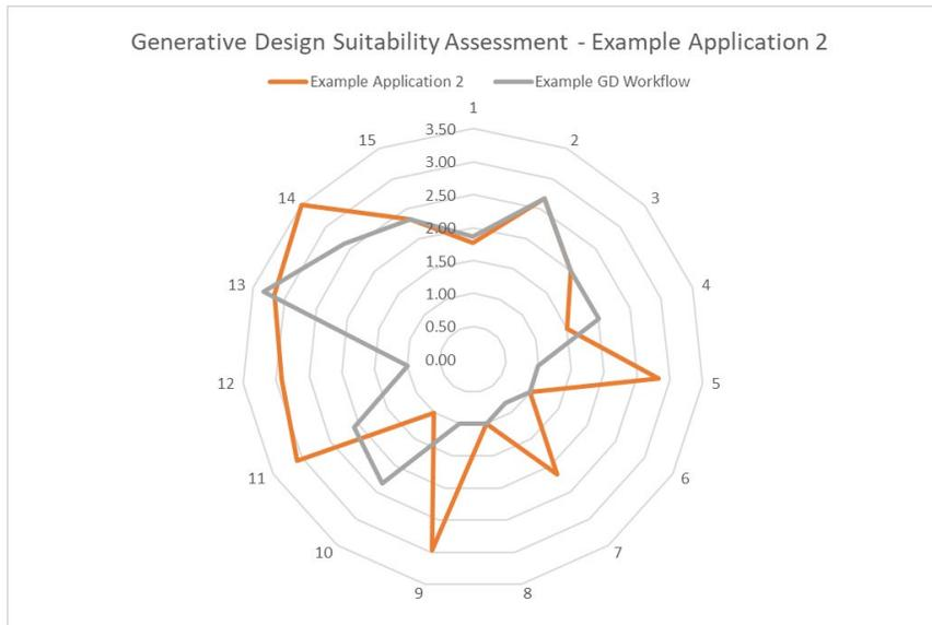
One possible approach for the Suitability Assessment is based on a quantifiable “Suitability Index.” A Suitability Index can be calculated for each Generative Design category of capability by dividing each applicable workflow capability rating by the corresponding application scenario requirements value.
