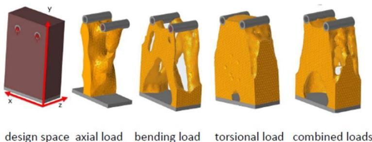
*Generative Design needs to work with design scenarios that include multiple load conditions to have a significant impact on the design process. These multiple load conditions are not encountered simultaneously but represent different use cases.*
