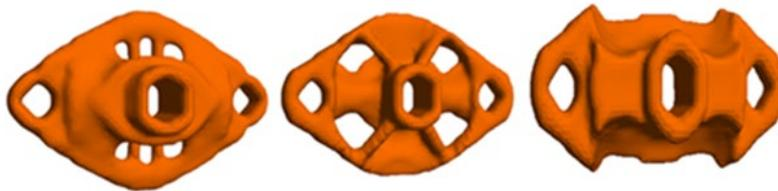
Different constraint combinations generate different designs
