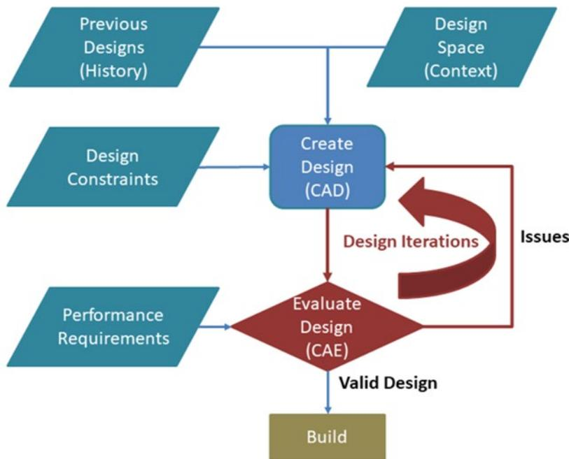
*The Generative Design process opens up the possibility thoroughly exploring the design space and discovering design concepts outside of previously accumulated proprietary knowledge.*
