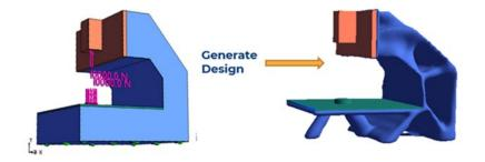
The second step toward the goal is enabling Generative Design of a multiple components simultaneously within an assembly context. The illustration below shows Generative Design of multiple components of the assembly performed simultaneously.
