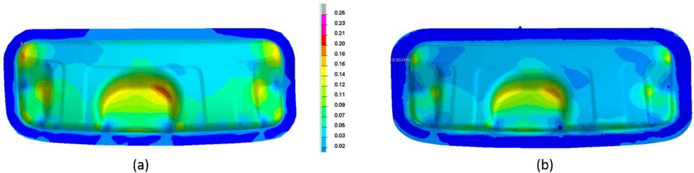
**Figure 3:** Customized die face of front hood reinforcement: (a) thinning color map before bead optimization; (b) thinning color map after bead optimization (improved formability)
