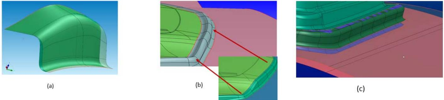
**Figure 4:** Examples of Die Starter optimization options: (a) changing automatically punch radius, (b) changing addendum by creating draw-bars, (c) changing automatically binder
