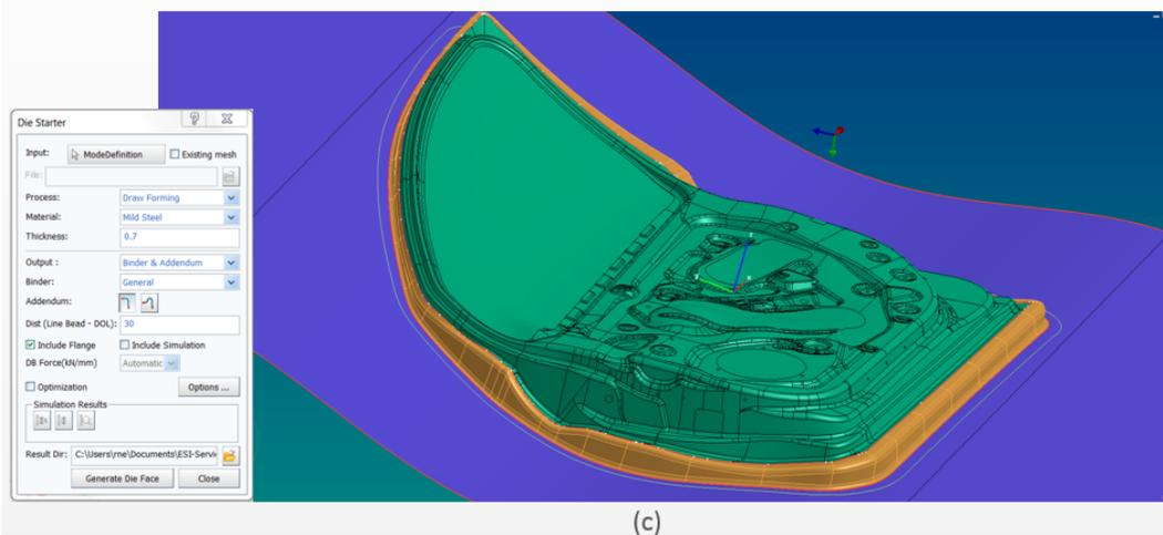
(c) Die Starter input deck and initial die face (binder, addendum, and bead center line) results
