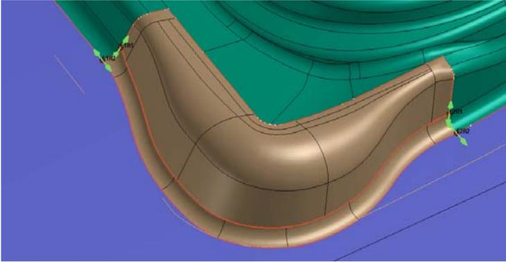
**Figure 2:** Manual local addendum modification (brown) in VDM based on Die Starter initial results
