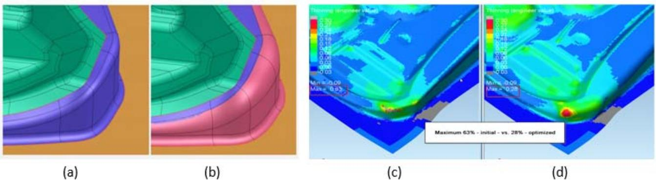
**Figure 8:** Die Starter hood inner rear corner: (a) Initial die face, (b) optimized die face, with (c), (d) thinning results comparison in PAM-STAMP
