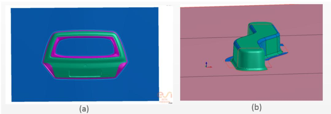
**Figure 6:** Example of Die Starter: (a) Liftgate outer with inner binder and addendum (Binder inner/outer in blue and addendum inner/outer in purple). (b) S-rail initial die face with part contour on binder
