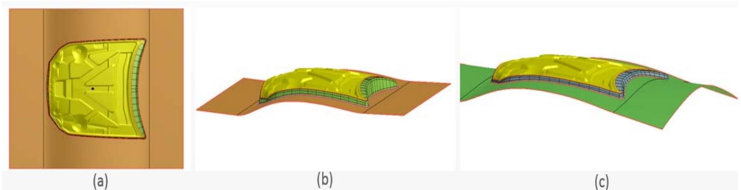
**Figure 5:** Example of Die Starter – Fully symmetrical die face of hood inner (a) with single curved binder (a) and double curved binder option (c)
