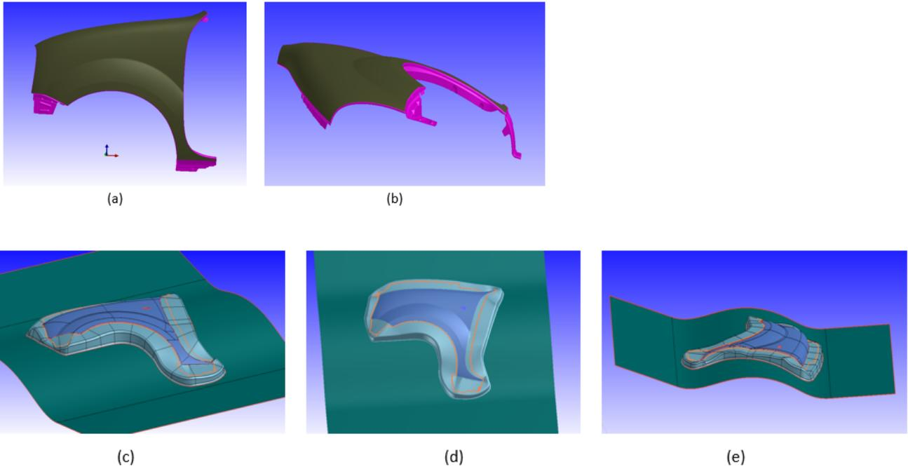
**Figure 7:** Die Starter fender initial die face with developed flanges: (a), (b) fender part with flanges; (c), (d), (e) initial die face with automatic developed flanges into addendum (developed trim line in orange)
