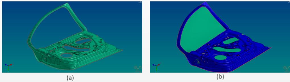
(a) Part geometry, (b) Die Starter part preparation (fill holes, smooth part outline)
