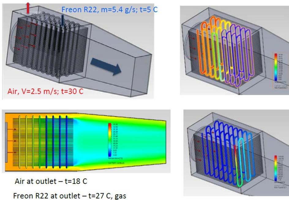
Figure 15: Air condition operation simulation
