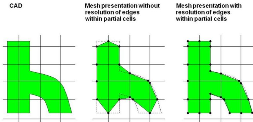
Figure 7: Mesh representation of CAD geometry with resolution of solid edges within partial cells.
