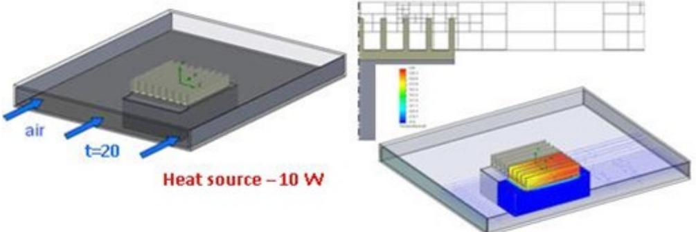
Figure 14: SOLIDWORKS Flow Simulation calculation using "Thin channel" technology.
