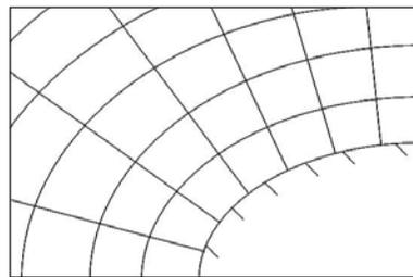
Figure 2: Structured body-fitted mesh
