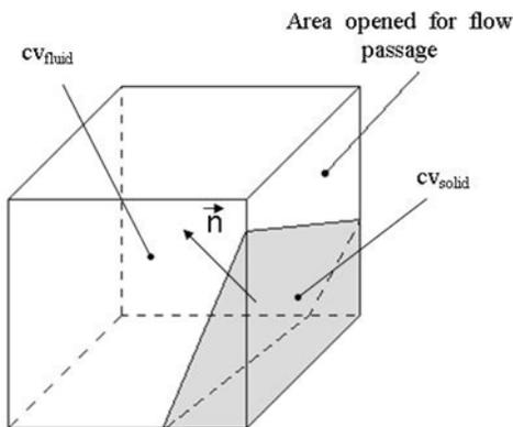
Figure 5: Partial cell in the simplest case and with 2 control volumes (CV) inside.
