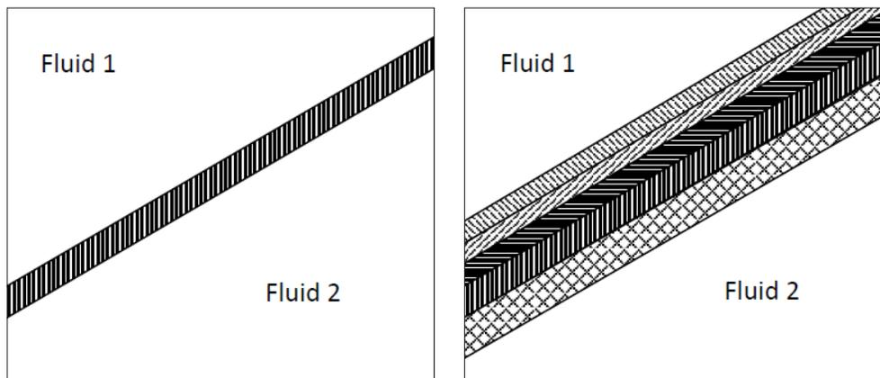
Figure 8-9: Partial cell with 3 control volumes (fluid-solid-fluid) in case of thin solid wall and partial cell with 7 control volumes in case of thin solid wall having inside 5 layers with different material properties.
