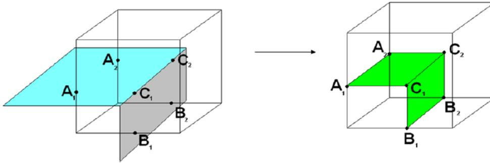
Figure 6: Representation of CAD geometry (left) in the partial cell (right) in case of 2 facets and solid edge inside one cell.
