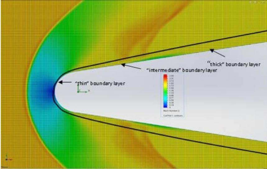
Figure 12: Mach Number flow field with "thin", "intermediate" and "thick" viscous boundary layer.
