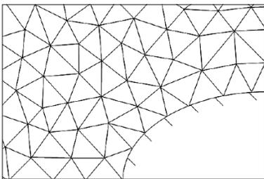
Figure 1: Unstructured body fitted mesh
