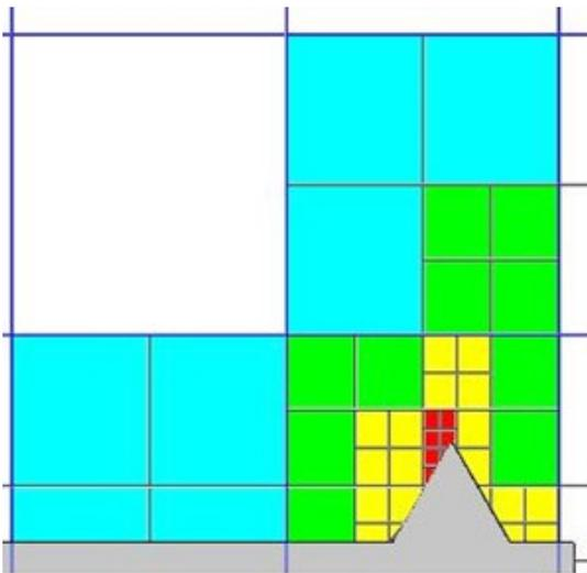
Figure 11: SOLIDWORKS Flow Simulation mesh after refinement.
