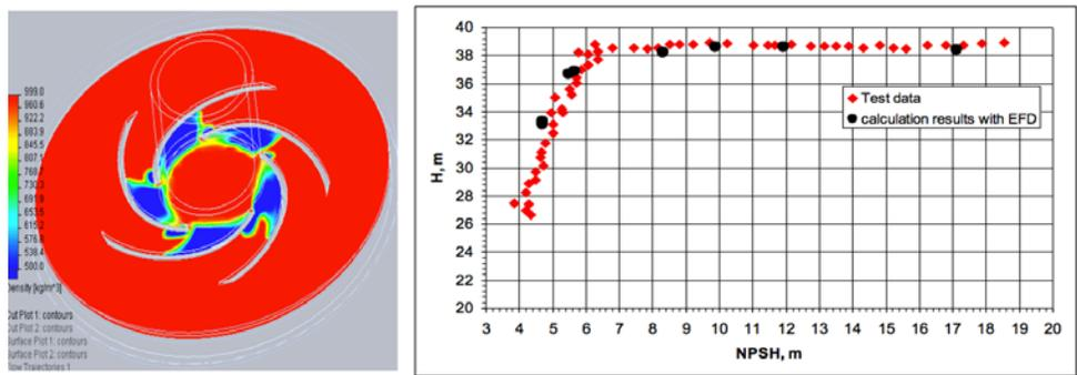
Figure 16. Calculation of cavitation in centrifugal pump.
