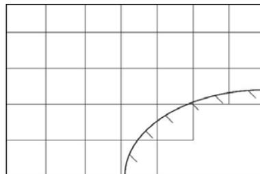
Figure 4: Structured Cartesian immersed-body mesh
