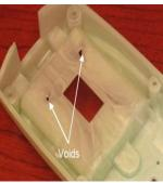
Thin section is surrounded by thick causing hesitation and voids
