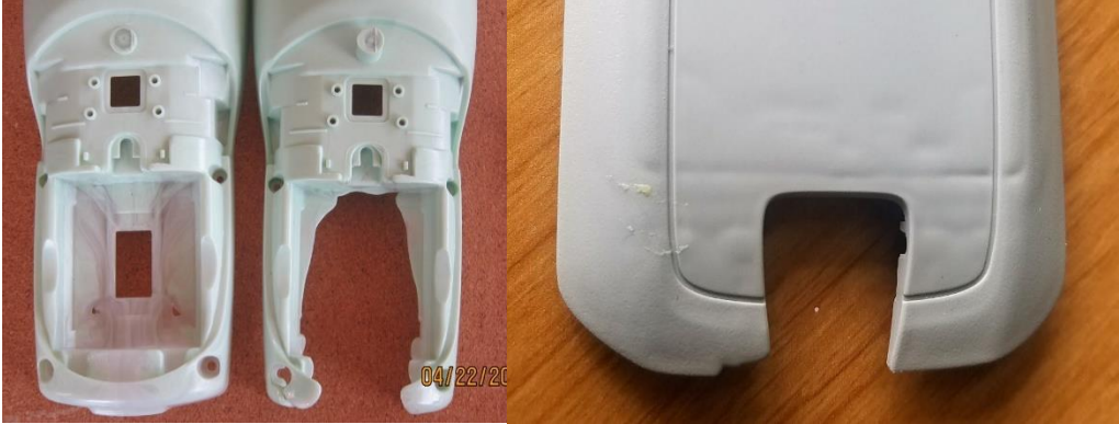
Figure 13: The flow marks and lack of filling (left) and ugly lines(right) in Thick sections
