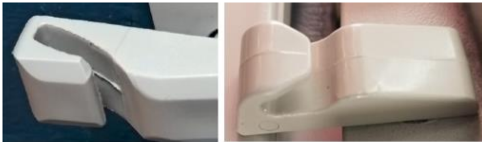
Figure 10: Ubiquitous latch for the folding tray table found on many commercial planes.
