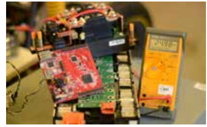
▲ The BMS master controller embedded hardware (red) sits on top of the BMS slave controller (green), which in turn sits on top of the battery demonstrator. The slave controller measures cell voltages and temperature, and executes the cell balancing strategy. The high-voltage battery disconnect (black box in rear) is responsible for connecting and disconnecting the battery from the load.
