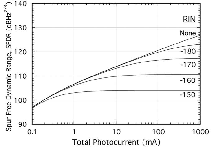
Fig. 7. SFDR of quadrature-biased MZM-based link as a function of photocurrent [98].
