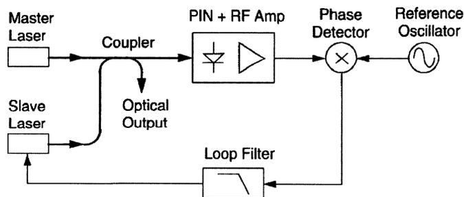
Fig. 4. OPLL microwave photonic transmitter [60].
