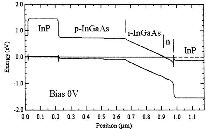
Fig. 6. Band diagram for surface illuminated designs PDA-PD [74].
