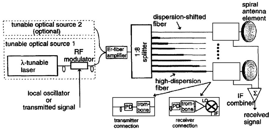
Fig. 11. True time-delay beam former using dispersive fiber [139].
