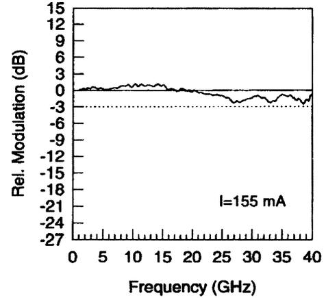
Fig. 1. Small-signal CW modulation response of 1.1  $\mu\text{m}$  wavelength quantum-well laser [23].
