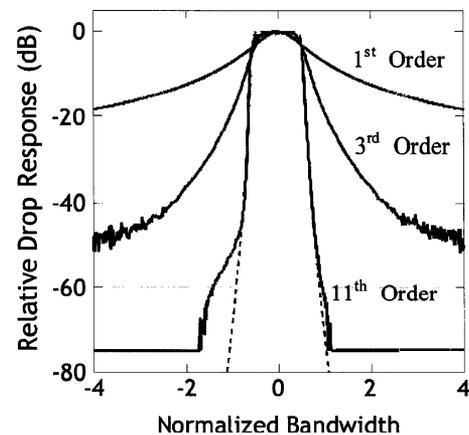
Fig. 10. Transmission characteristics of microring-resonator filter as a function of order [125]. Bandwidth normalized to the  $-3$  dB filter bandwidth.
