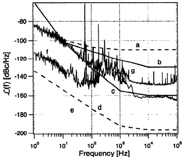
Fig. 12. Comparison of phase-noise spectrum at 1 GHz between (a) low-noise quartz oscillator, (b) low-noise RF/microwave synthesizer, (c) sapphire loaded cavity oscillator, (d) projected for Ca optical standard, (e) projected for visible laser that serves as a reference for  $\text{Hg}^+$  optical standard, (f) optical pulse train output of femtosecond laser synthesizer, and (g) microwave electronic output of femtosecond laser synthesizer [150].
