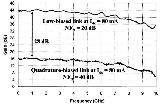
Fig. 2. Measured link gain against frequency for externally modulated quadrature-biased and low-biased (suppressed carrier) links [32].
