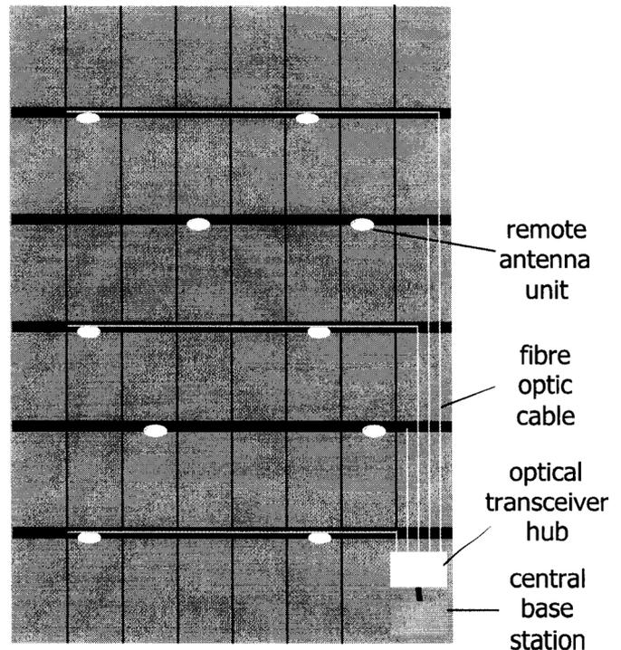
Fig. 8. In-building fiber distributed antenna system.
