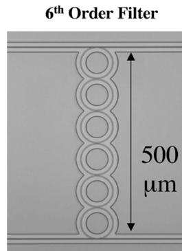
Fig. 9. Sixth-order microring-resonator filter [125].
