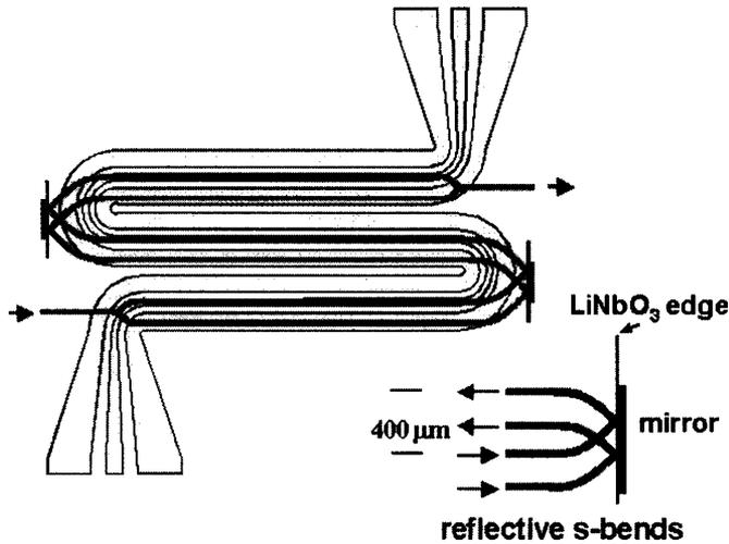
Fig. 3. Multipass lithium-niobate modulator design [33].
