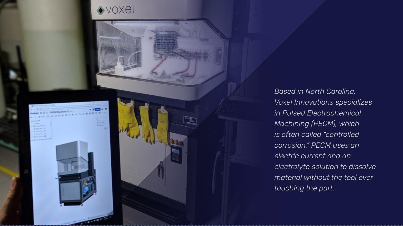
*Based in North Carolina, Voxcel Innovations specializes in Pulsed Electrochemical Machining (PECM), which is often called “controlled corrosion.” PECM uses an electric current and an electrolyte solution to dissolve material without the tool ever touching the part.*
