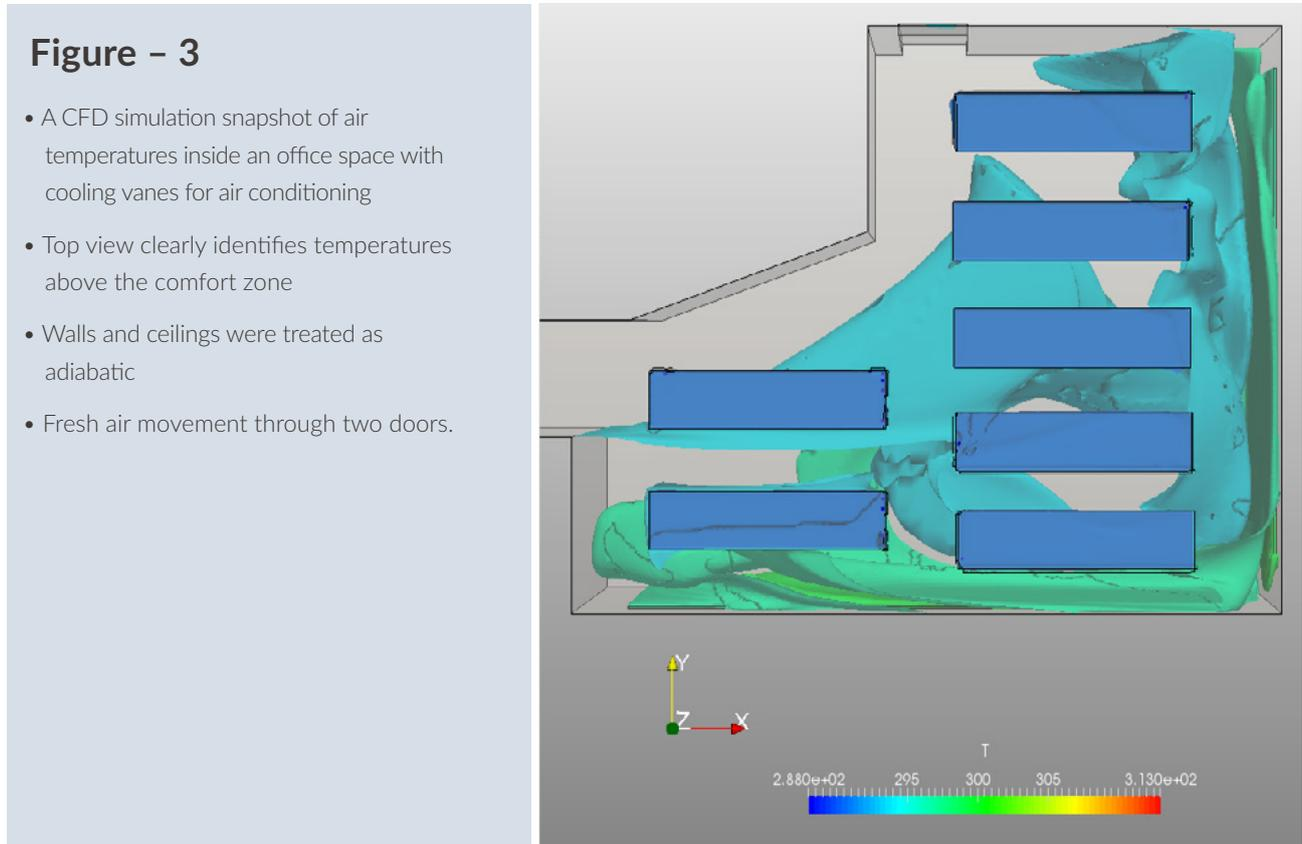
**Figure – 3** is a plan-view snapshot of the same **steady state simulation** carried out on SimScale, showing temperature distribution along the length and breadth of the conditioned space, blue being the coolest zone and red/orange as the hottest zone. This top view has again highlighted the weakness of the HVAC system design to create comfortable air conditioning close to windows.
