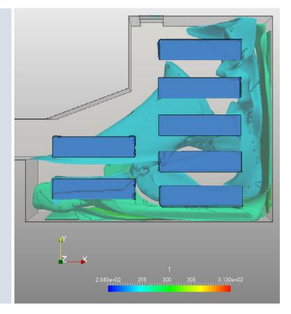
**Figure – 3** is a plan-view snapshot of the same **steady state simulation** carried out on SimScale, showing temperature distribution along the length and breadth of the conditioned space, blue being the coolest zone and red/orange as the hottest zone. This top view has again highlighted the weakness of the HVAC system design to create comfortable air conditioning close to windows.
