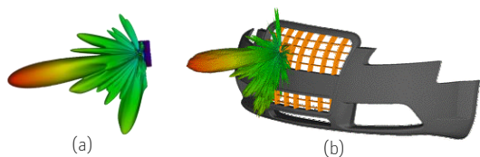
Figure 7. (a) Pattern of radar in free space (b) Changed pattern when same radar is installed in a vehicle fascia.
