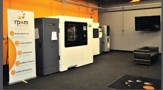
Three of rp+m's FDM additive manufacturing machines.
