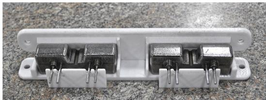
Even simple CMM fixtures can save hours in the inspection process.
