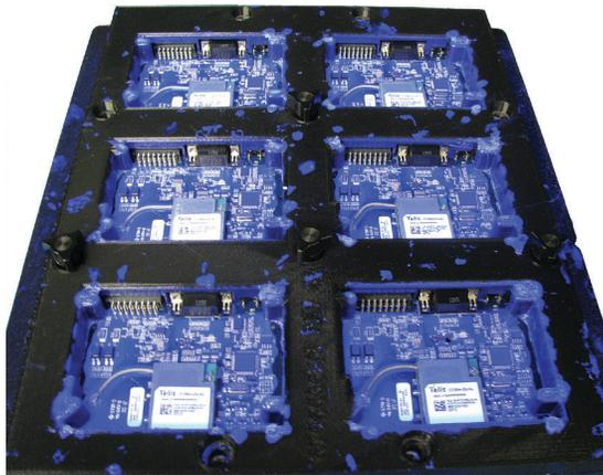
FDM hybrid mask (black) shields PCB components from conformal coating (blue under ultraviolet light).
