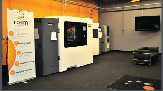
Three of rp+m's FDM additive manufacturing machines.
