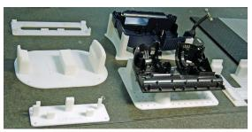
Even simple CMM fixtures can save hours in the inspection process.
