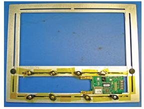
Machined carrier with manually applied tape for masking.
