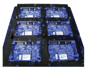
FDM hybrid mask (black) shields PCB components from conformal coating (blue under ultraviolet light).
