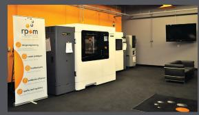
Three of rp+m's FDM additive manufacturing machines.
