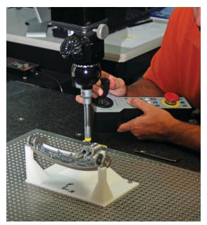
Using AM fixtures, Oreck completes CMM programming before first articles arrive.
