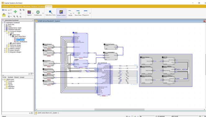
Figure 6: The E/E architecture can be represented as a network view with ECUs and communication busses, as a platform topology, or functional view.
