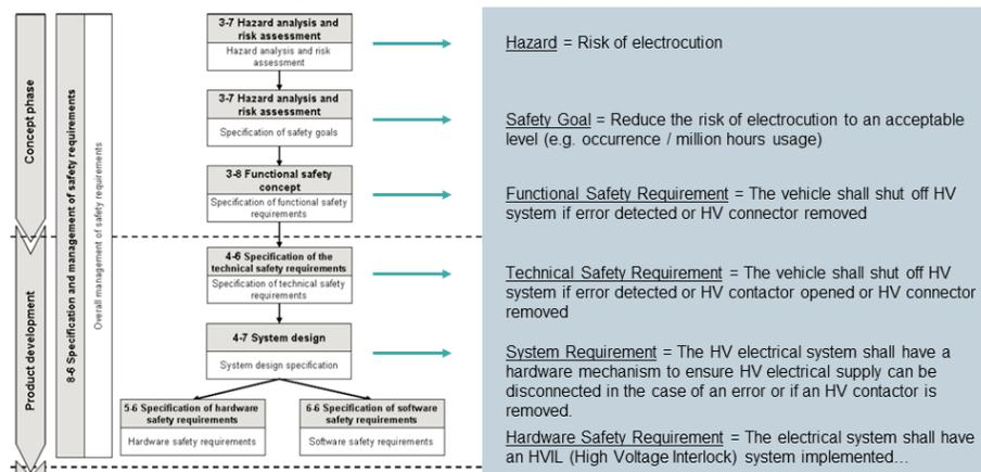
Figure 7: An example illustrating the additional safety planning needed for an EV. Image source: (International Standards Organization, 2018).
