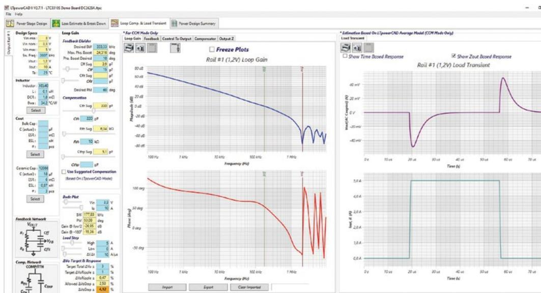
Figure 7. Setting the control loop with LTpowerCAD.
