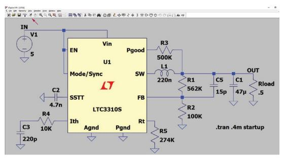
Figure 10. Simulation circuit of an LTC3310S using LTspice.
