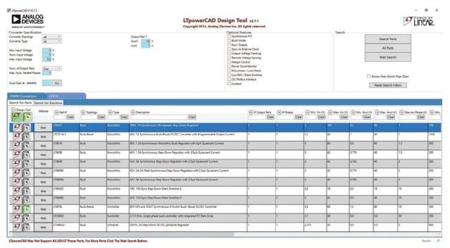
$\label{thm:continuous} \textit{Figure 3. Searching for suitable switching regulator ICs with LTpowerCAD.}$
