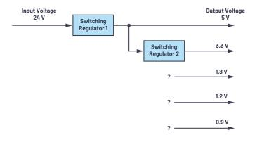
Figure 1. Creating a power supply architecture.
