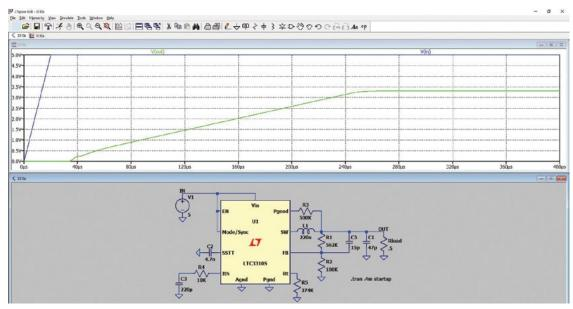
Figure 11. Simulation result of an LTC3310S circuit using LTspice.
