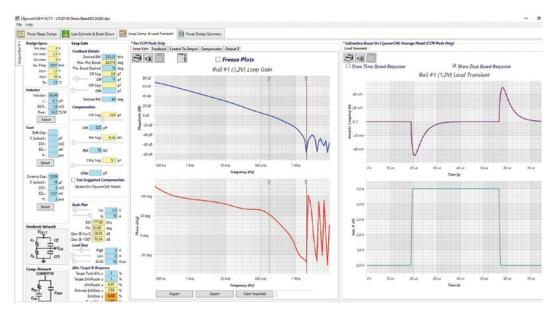
${\it Figure 7. Setting the control loop with LTpowerCAD.}\\$
