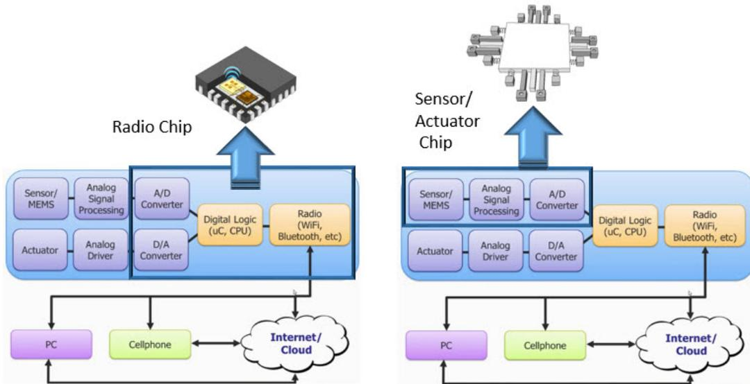
Figure 2: Converging functional blocks in order to create a multi-functional chip.
