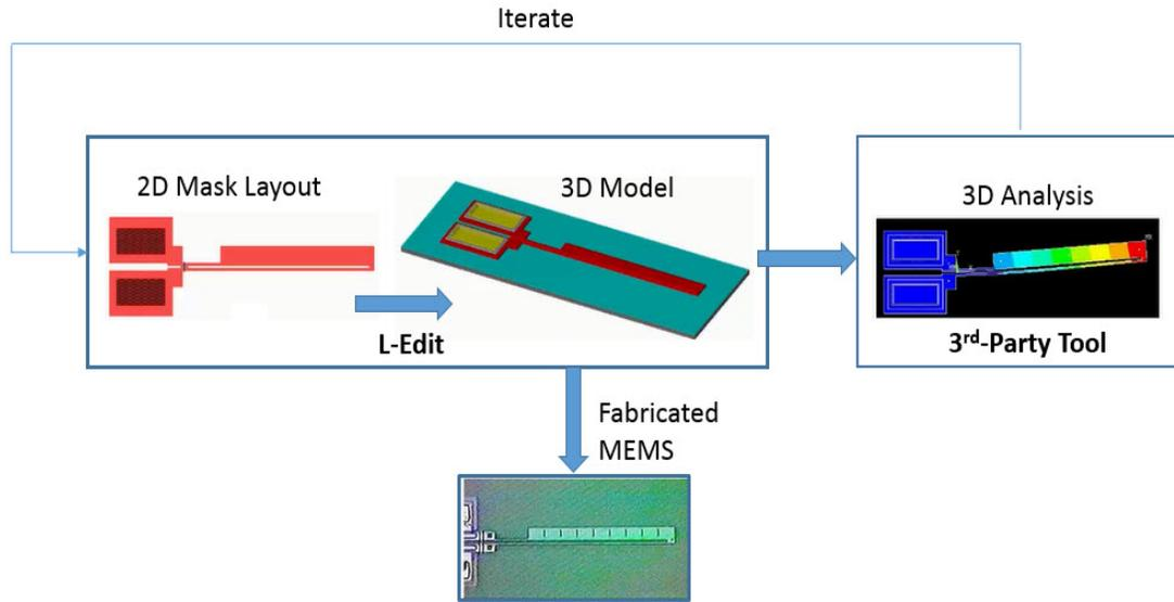
Figure 7: The mask-forward MEMS design flow.
