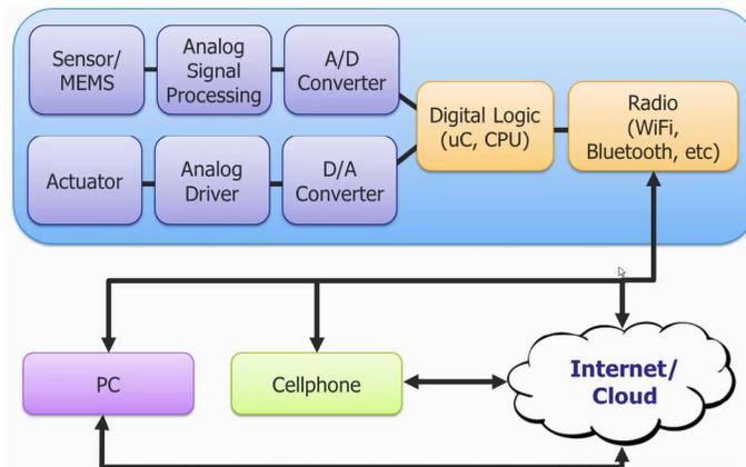
Figure 1: A typical IoT device.
