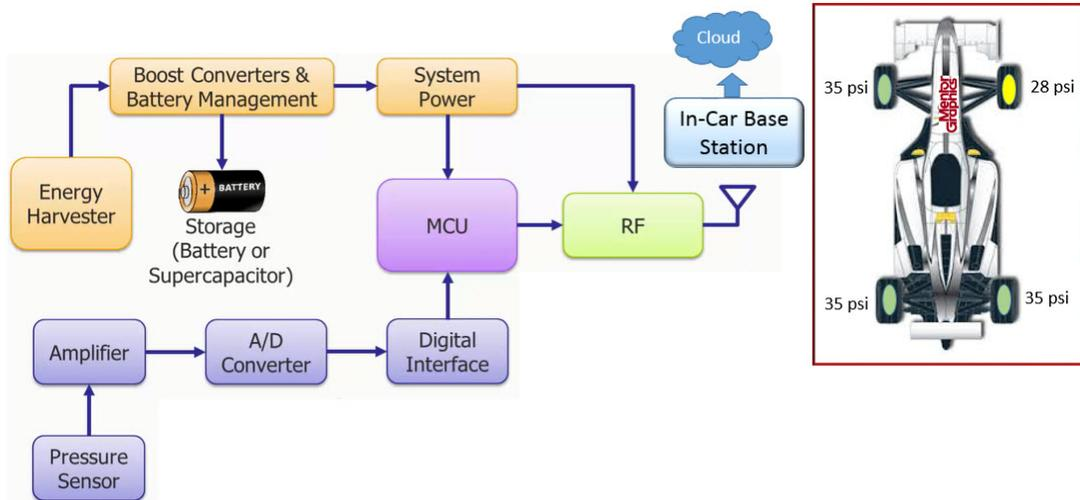
Figure 3: A racing team tire pressure monitoring system.
