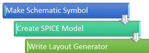
Figure 5: An overview of the process for making your own primitives.
