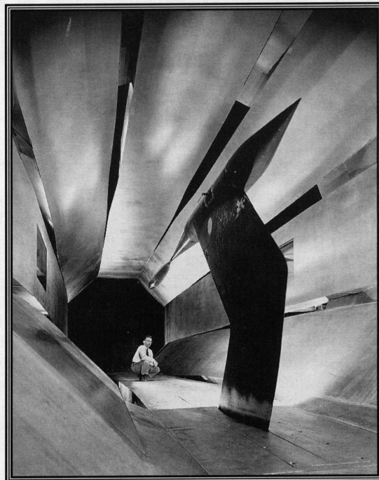
The secret to building a transonic wind tunnel—slots in the throat of the test section. Taub's photograph was marked "Top Secret" for a number of years.
