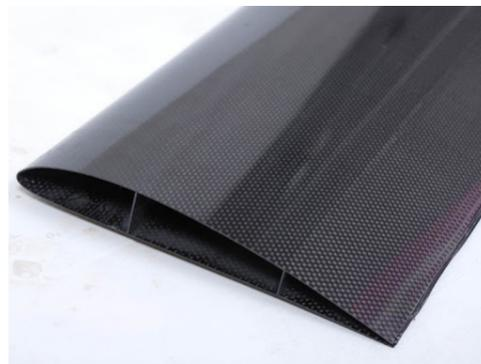
**Carbon fiber construction makes the OA-2H lighter and more durable than other airframes**
