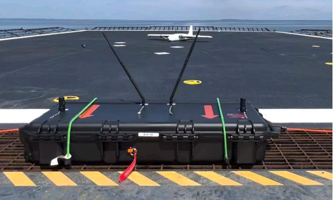
Offshore Aviation autonomous ship landing system, "Pathfinder", allows aircraft to find a moving vessel, setup an approach and land autonomously on a designated flight deck.
