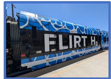
FLIRT H2 - Power unit containing the batteries and fuel cells
