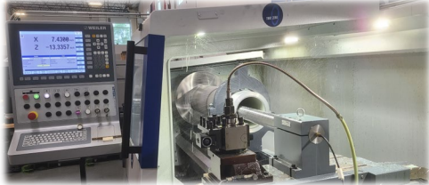
Parts fabrication on computer-controlled lathe.
