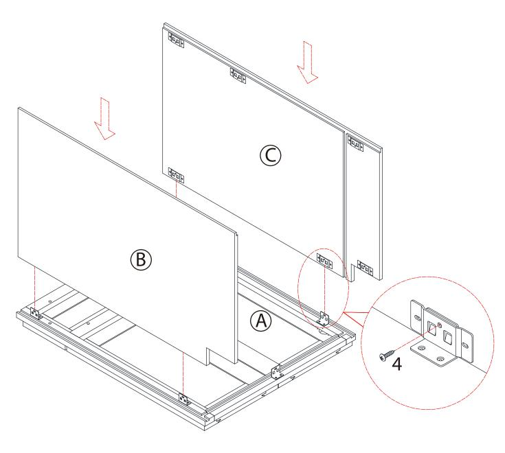
**PRO TIP:** When placing side panels into brackets, slide female end over male going into slot over the face frame. While doing this, if you slightly angle the panel as the bracket makes female to male connection, it helps lock the fasteners into the groove.
