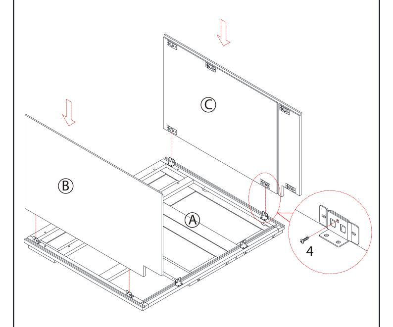
**PRO TIP**: When placing side panels into brackets, slide female end over male going into slot over the face frame. While doing this, if you slightly angle the panel as the bracket makes female to male connection, it helps lock the fasteners into the groove.
