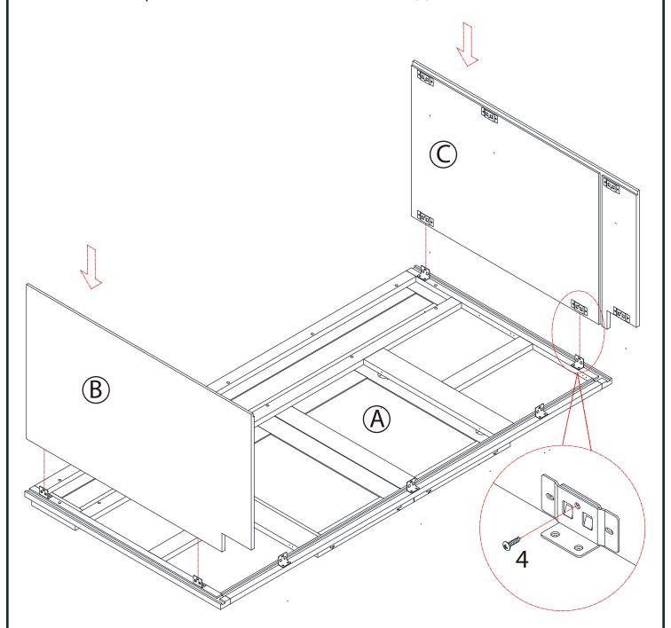
**PRO TIP**: When placing side panels into brackets, slide female end over male going into slot over the face frame. While doing this, if you slightly angle the panel as the bracket makes female to male connection, it helps lock the fasteners into the groove.
