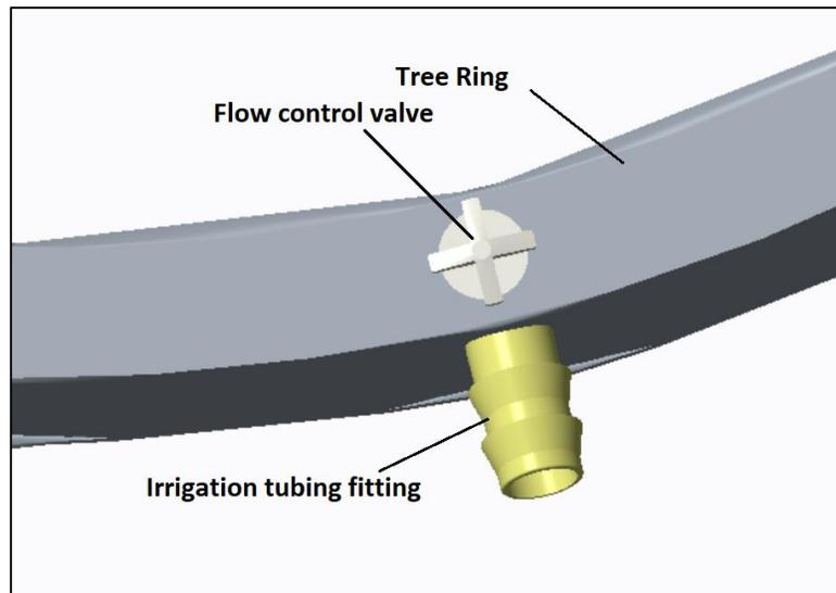
TreeHydrant is a revolutionary water delivery and conservation system for commercial, residential and agricultural applications. The Original Inventor of past tree rings introduces a ring with innovative design and functions unlike any other in the market!
