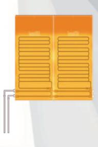
Filling the system should be done using a filling and flushing unit (vacuum-based). If a filling station is not available, you can adjust the valves installed in each panel. To check the operation of the system, you can also use a thermal imaging camera aimed at the surface of the operating panels. Adjustment can also be carried out using an infrared thermometer, measuring the panel temperatures.
