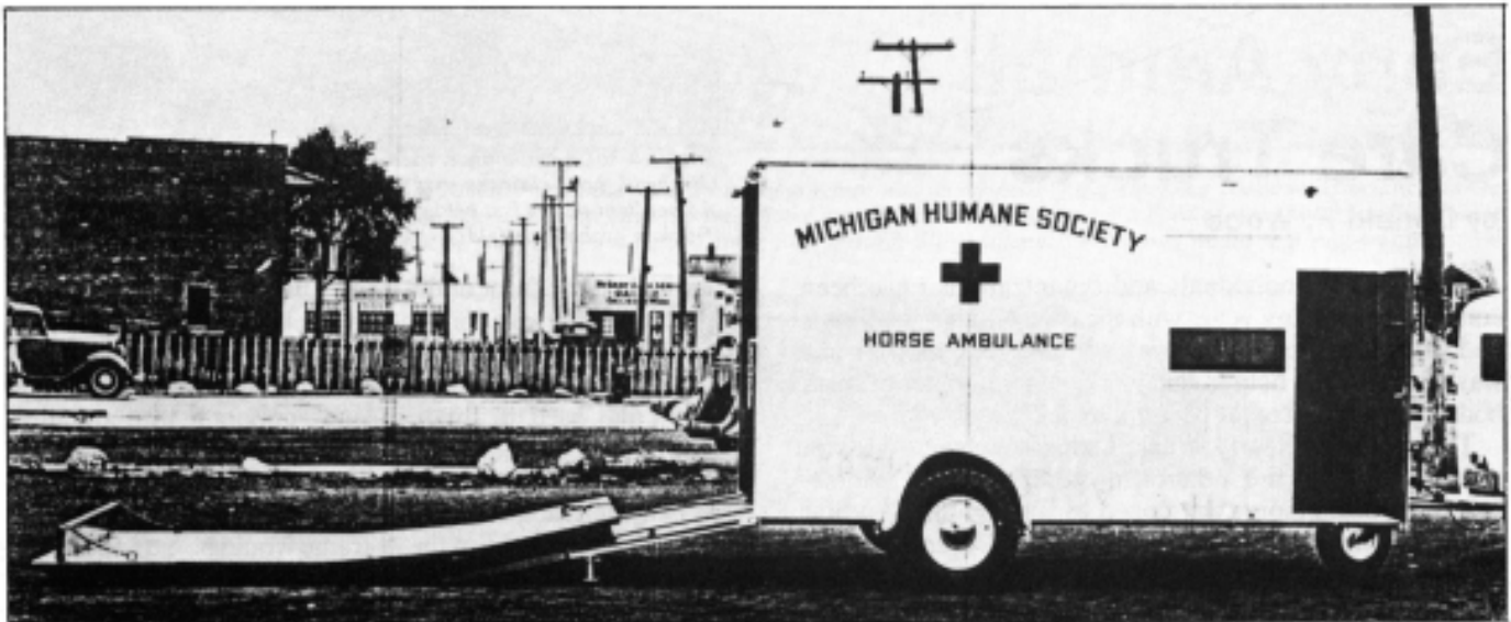
Above and Below: This mid-30's Ford panel truck with three-wheel trailer was used in Detroit as a horse ambulance. A cable and winch could be used to pull the mattress up the ramp.
