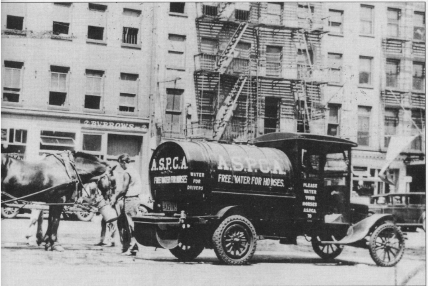
Above: This Ford TT was used in cities for giving work horses an opportunity to drink. Ice water was carried to be given to the teamsters, and act as an incentive for them to stop to let their teams drink. Holes in tires were to increase cushioning effect. Below: This truck was used by the Royal Society for the Prevention of Cruelty to Animals during World War I, and is shown at a veterinary hospital in France in 1916.
