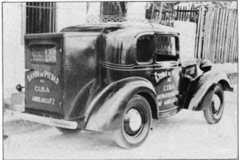
This small animal ambulance was used in Cuba, before World War II. Vehicle is an American Bantam with an extra compartment added to the rear.
