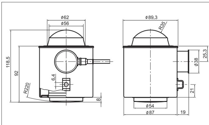
Truck scale load cell PR 6221
