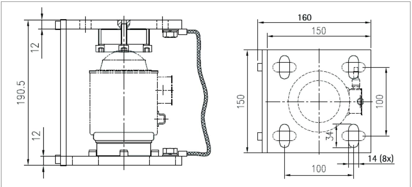
Truck scale load cell PR 6221 in mounting kit PR 6021/01N
