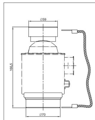
Truck scale load cell PR 6221 with standard load disc kit PR 6021/00N
