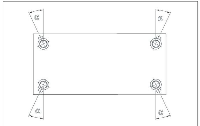
To reduce the number of displacement errors, the adjustment chambers of the load cell must be positioned at an angle of  $\alpha = 20$  to  $30^\circ$ .
