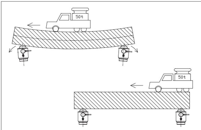
Load-induced deflection of the scales can result in inaccurate measurements. The PR 6221 therefore has a patented displacement error reduction mechanism.
