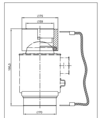
Truck scale load cell PR 6221 with turbo load disc ..04N\*
