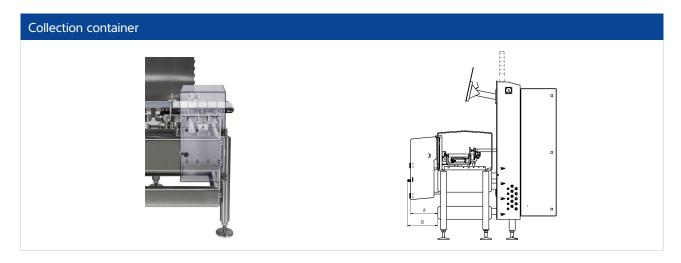
The scale drawing shows Flexus® with a collection container (optional), which is made from plastic (option SSC: the plastic is additional reinforced) or stainless steel – both versions have different dimensions.
