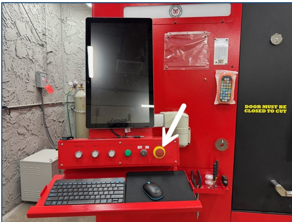
Figure 1. The E-stop is the red knob on the right end of the operator console (arrow). Release it by turning it clockwise until it pops out.
