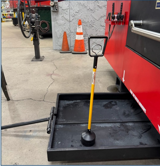
Figure 35. A catch tray pulled out, with the large yellow magnet standing in it. The tray handle is folded down: leave it tucked in so it is not a trip hazard.
