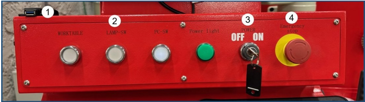
Figure 9. The operator console: 1 = USB slot (left end), 2 = LAMP-SW, 3 = keyed power switch (O = off, I = on), 4 = Emergency stop.
