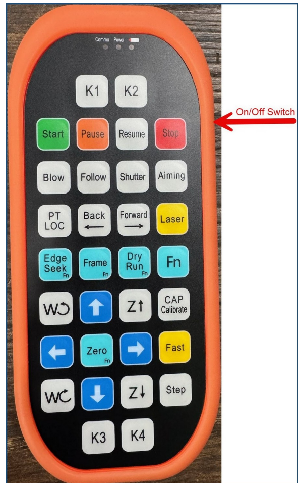
Figure 5. The remote control. The On/Off switch is on the side (arrow). Edge Seek, Frame, Dry Run, and Zero are used together with the Fn key; K4 is at the bottom right.
