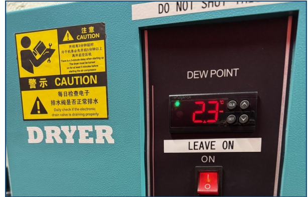
Figure 32. The dryer's DEW POINT display, here reading 2.3 °C. Below 3 °C is ready to cut. The dryer switch stays on; cutters never touch it.
