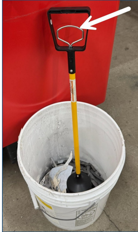
Figure 36. Emptying the yellow magnet over the scrap bucket: pull the silver release handle inside the black handle (arrow) and the metal drops off.
