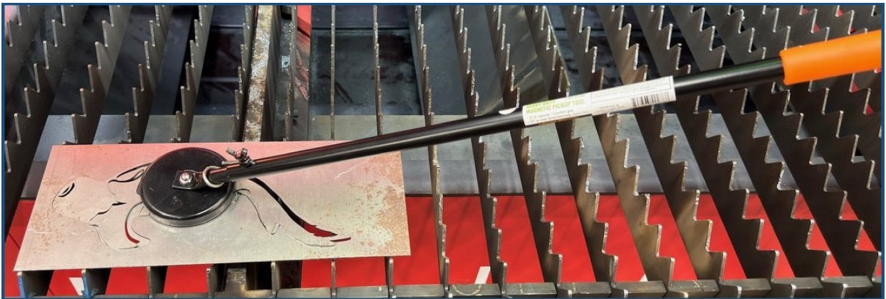
Figure 33. The medium magnet (black shaft, orange handle) lifting a cut part without disturbing the sheet.
