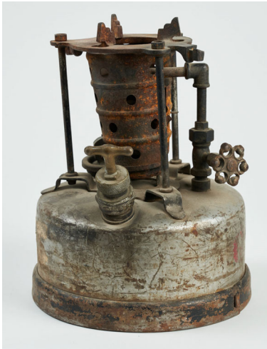
Blow Pot for engine oil in the 1920/1930's for Bush Pilots or Cold weather
