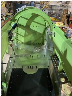
Within a month we had found most them, and got to work fitting them to the fuselage. We also installed pulleys, the seat, interior panels, the flap mechanism, fuel selector and other various components.
