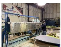
weeks that we have been able to see all the months of work pay off as we have been able to rivet in the floor and have nearly completed installing the side skins.
