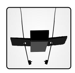
Using counterclockwise rotation, remove your computer from the AEROVED mount. Place the mount on top of the taped areas on the extensions and install the 2 straps from the bottom of the mount. Make sure that the head of each strap is facing away from the extension bar that it's being mounted on (See image ABOVE).
