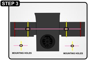
Use the measurements from <a href="Step 1">Step 1</a> to mark the locations of the inner and outer edges on the mount. Measure the width of the wings and mark the center location where the mounting holes are. Using a 6mm drill bit, drill two mounting holes at this marked location.
