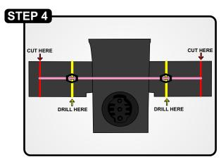
Cut the extra materials off of the wings using a tool such as a hacksaw. Before you make the cuts, make sure the distance between the two outer lines on the mount match the distance between the outer edges of your aero extension from <a href="Step 2.">Step 2.</a>
