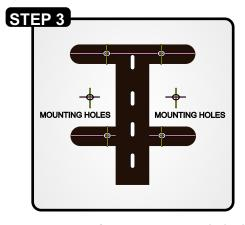
Use the measurements from <u>Step 2</u> to mark the locations of the inner and outer edges on the mount. Measure the width of the wings and mark the center location where the mounting holes are. Using a 6mm drill bit, drill four holes at this marked location.
