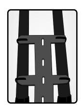
Place the bottle mount on top of the taped areas on the extensions and install the 4 straps from the bottom of the mount. Make sure that the head of each strap is facing away from the extension bar that it's being mounted on (See image ABOVE).
