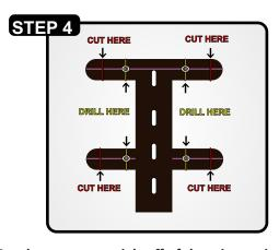
Cut the extra materials off of the wings using a tool such as a hacksaw. Before you make the cuts, make sure the distance between the two outer lines on the mount match the distance between the outer edges of your aero extensions from <a href="Step 2">Step 2</a>.
