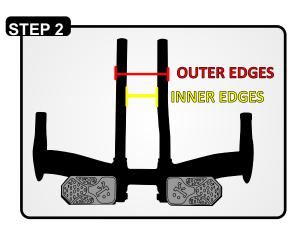
Measure the distance between inner and outer edges of your aero extensions.
