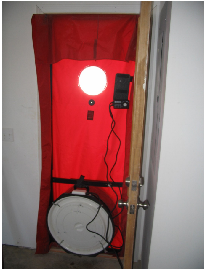
A blower door set up and ready to test a house
