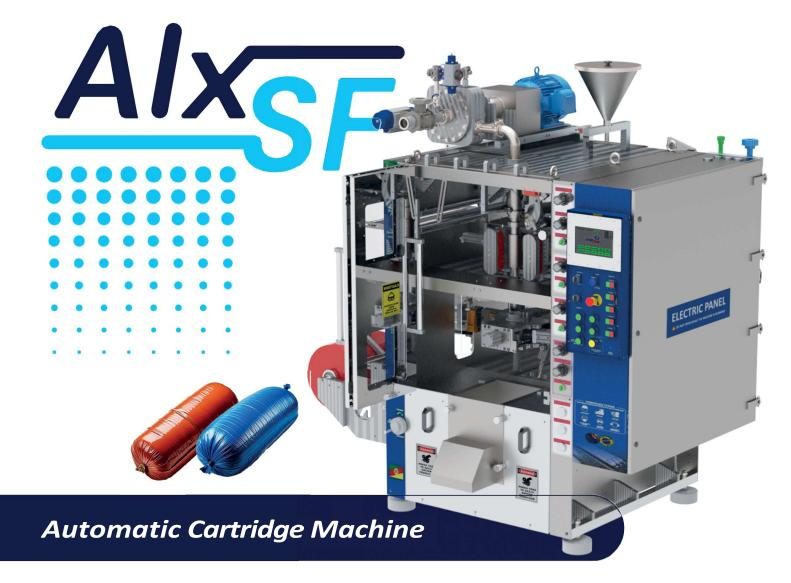
The ALX-S produces ultra low-cost packages at speeds up to 120 packages per minute in diameters ranging from 22-150mm. Clips are formed with a state-of-the-art continuous motion clipping table. The clipping table uses spooled wire to reduce package costs vs pre-formed clips. Roll-stock film is sealed by heat or glue extrusion depending on packaging needs.
