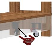
After inserting the 4 wood screws, turn your part back on its legs and <u>then</u> remove the 4 red wheel locks. The casters are now ready to use.
