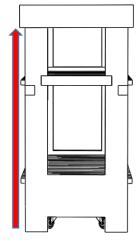
*If one side is picked up unevenly and 1 caster does not engage, raise that corner 1" and then lower down.*
