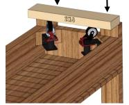
Before mounting the casters, hold a straight piece (such as a 2x4) across the legs. Peel the mounting tape and apply the caster to your part. <u>Please Note</u>, the bottom of the caster wheel should slightly touch, the 2x4. Remove the 2x4, drill 4 pilot holes and then insert the 4 wood screws (do not remove the wheel locks yet).
