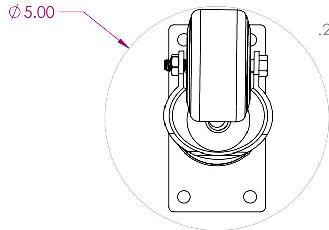
**ALLOW 5" OF CLEARANCE FOR THE SWIVEL RADIUS OF THE WHEEL.**
