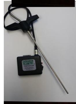
**HUMIDITY SENSORS / PSYCHROMETRIC SENSOR.** The Humidity Sensor measures three parameters and calculates several others. Sensor is available in three standard shaft lengths, 5", 16", and 48". 5" type has a magnet to hold it against the duct when inserted through a 3/8" hole.
