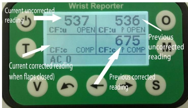
10. A compensated reading may be stored when continuous backpressure compensated readings are being displayed at the lower left. Whenever satisfied, press “S” or press the Thumbswitch to record the two values. A small “s” will be shown beneath the two values to indicate they have been stored. In addition, the sequence number next to the Memory Group letters will increment.
