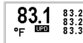
**Store/Stats Screen:** The Store/Stats screen displays the most recent reading. The memory group and the sequence number within the memory group are displayed at the bottom of the screen. The minimum, maximum, and average statistics associated with the current memory group are displayed on the right of the screen.
