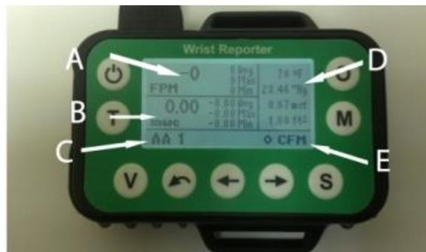
**Velocity Store/Stats Screen:** Shows latest reading in large numbers in the center of the screen. Average maximum and minimum are shown on the right side of the screen. Group and number of stored readings can be seen on the bottom left and average CFM is displayed on
