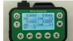
If more than four sensors are linked to the Wrist Reporter, they can be quickly and easily viewed in two Split Screens back-to-back. The first shows Sensors 1-4, and the second shows Sensors 5-8. The ESC key is used to flip back and forth between the two screens.
