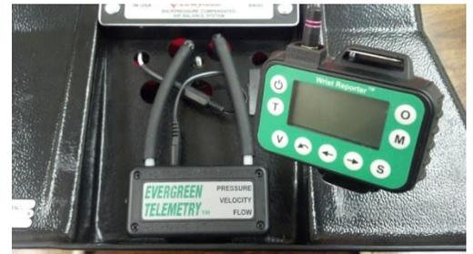
1. Remove the digital meter from its normal mounting position. Install the two adhesive-backed Velcro pads as shown in the photo. Install the corresponding Velcro pads on the bottom of the Evergreen Pressure Module. The magnet can be installed on the upper right to support the Evergreen Temperature Module.
