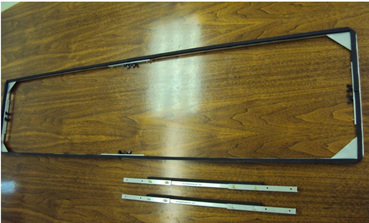
At each junction the connecting bridge fits onto four threaded inserts. Only the two closest to the junction need be secured by nuts—the other two function as guide pins. In addition to the traditional brass knurled nut, the user has the option of plastic wing nuts. Lock washers are provided to help keep the nuts from loosening.
