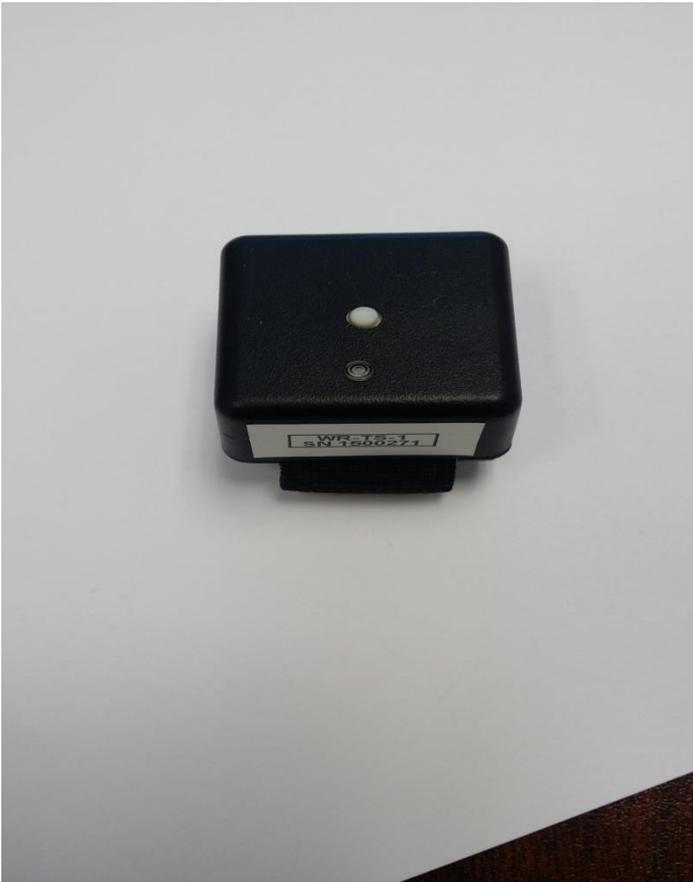
The Thumbswitch makes it easier to store readings. Pushing the button causes the same action as pressing S on the Wrist Reporter. It can be worn on a finger and activated by a small motion of a thumb or other finger. It eliminates the need to reach over to the Wrist Reporter with the opposite hand/arm.
