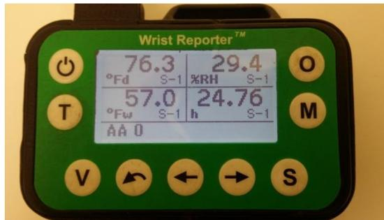
Press the arrow keys to highlight one of the four quadrants. Press S to select that quadrant for change. Press the arrow keys to change the parameter displayed. Press S to confirm that parameter for that quadrant. Press the arrow keys to highlight a different quadrant for change. Etc. When satisfied with the display format, press V to display measurements.
