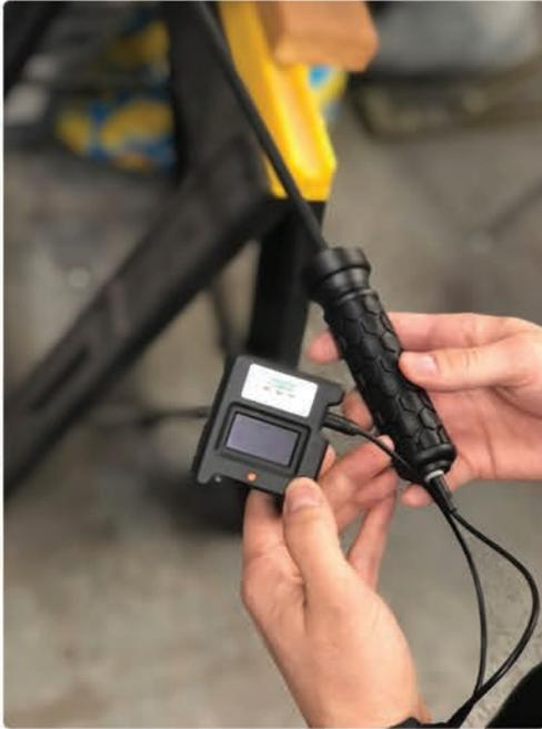
Meter-Sensors have an on-board display and can be used as a stand-alone unit when taking quick readings.
