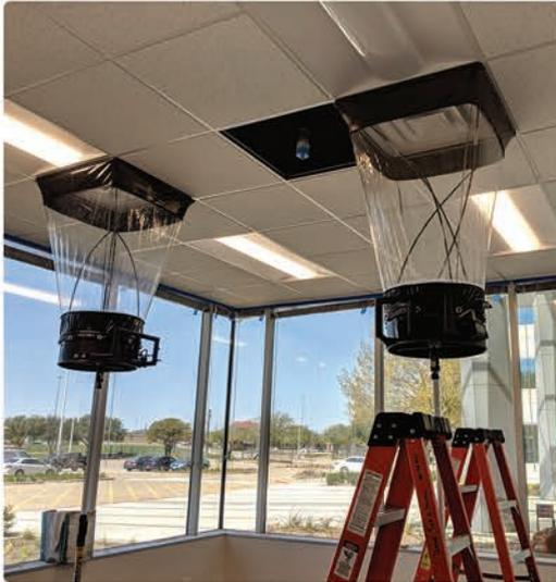
Evergreen Telemetry's line of capture hoods offer different options for different applications. View up to 4 real-time, continuous, wireless readings from different locations. With the magnet frame, you can make damper adjustments, with only one trip up the ladder. Faster, Easier, Safer!
